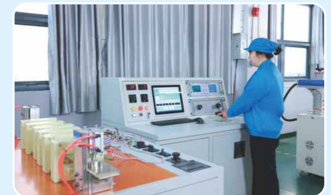
Electric current transformer calibration station
