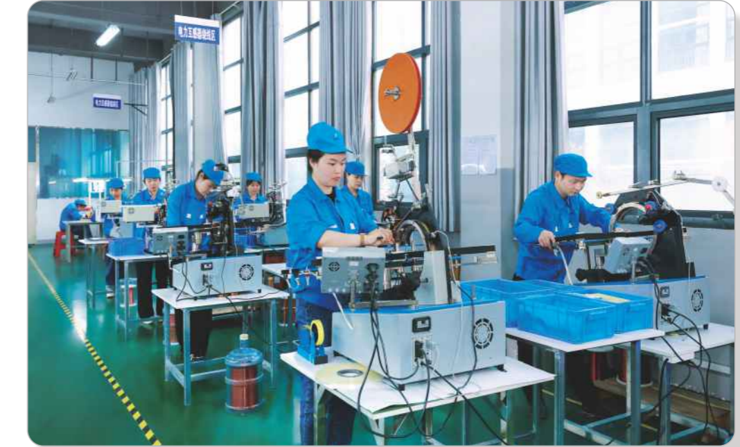
Electric current transformer winding
