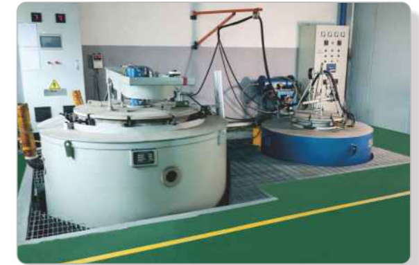
Silicon strip core heat treatment furnace
