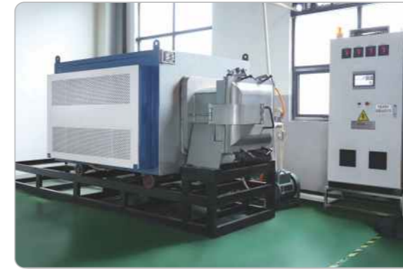
Nano-crystalline core heat treatment furnace
