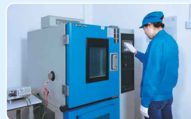
High&low temperature and humidity chamber
